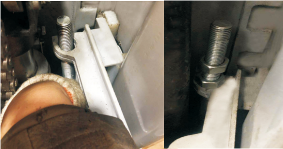
Fig7-5 Fix on the hole and screw up the screws , same installation of two side
