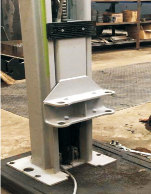
Fig6 Put up the pillars and lifting slide table to 400mm -500 mm high(two pillars is the same)
