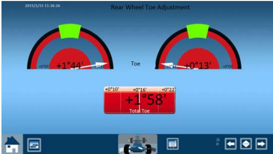
Individual adjustment of rear wheel Toe
