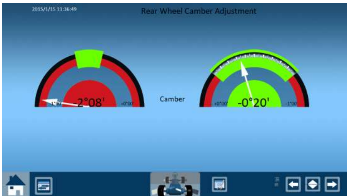
Individual adjustment of rear wheel Camber
