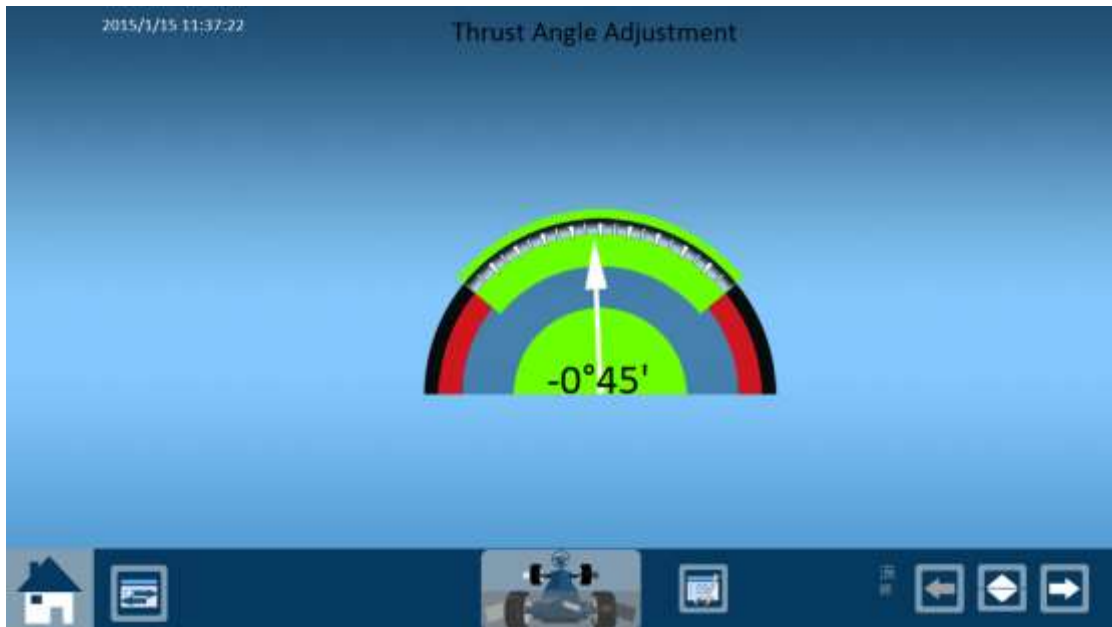
Individual adjustment of rear wheel thrust angle
