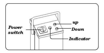
When the power supplied, turn the *POWER SWITCH* clockwise while the machine is on standby and an *INDICATOR* will show.
