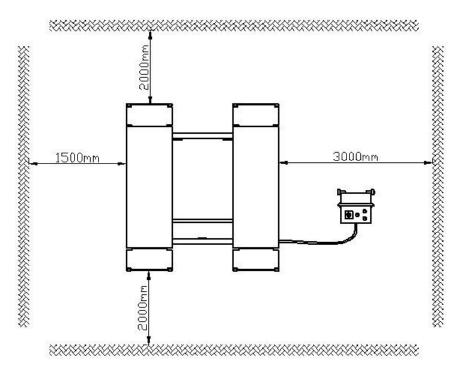
These measurements are also the machine working range. Persons other than specially trained and authorized operators are expressly forbidden to enter this area,
