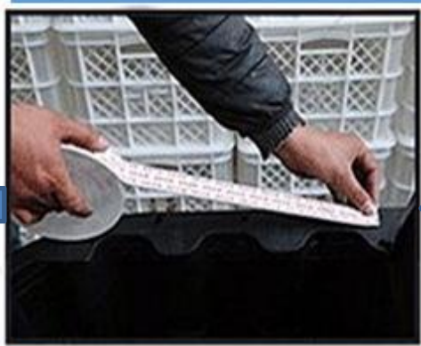
5. Sealing tape on the edge of the bottom tank
